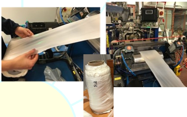
Flat die extrusion of PLA (top) and flat die extruded film roll based on plasticized PLA blends (bottom).
